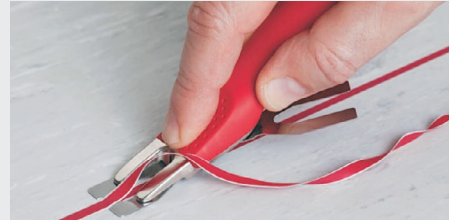
Swing slide out for trimming cut
