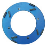
Grinding disc blue HB grit 30/40 Hard bond for soft, abrasive to medium-hard surfaces, e.g. screeds
